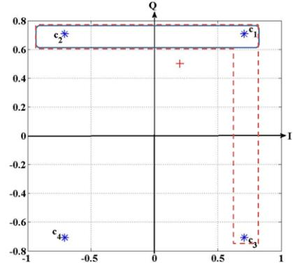
Fig. 3. Complex plane with received modulation symbol and considered candidate transmit symbols
