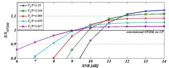
Fig. 7. Relative spectral efficiency of the proposed system applying FTN
