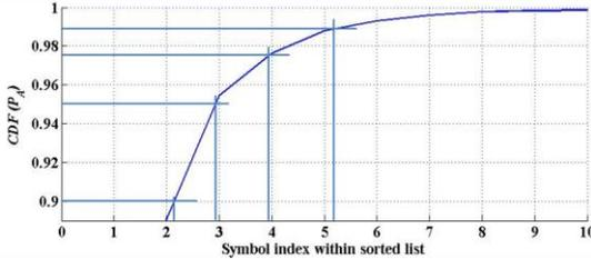
Fig. 4. Strategy to determine  $K''_{\text{sctr}}$  for a targeted detection probability  $P_A$  ( $\text{SNR} = 10\text{dB}$ ,  $T_o/T = 1.085$ )
