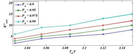
Fig. 5c.  $K''_{\text{sctr}}$  for DFT based preselection using the distance to the closest decision threshold as reliability measure
