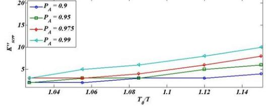
Fig. 5a.  $K''_{\text{sctr}}$  for MMSE based preselection using the distance to the closest decision threshold as reliability measure
