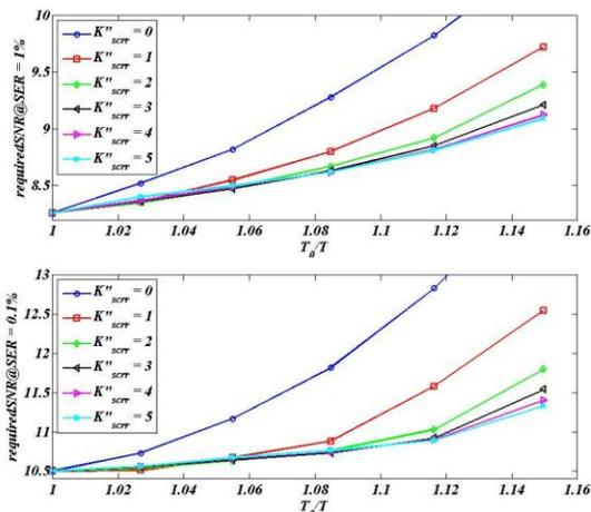
Fig. 6. Required SNR to achieve a given SER (1%, 0.1%) depending on the grade of overlap for various  $K''_{serr}$
