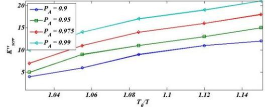
Fig. 5d.  $K''_{\text{sctr}}$  for DFT based preselection using the distance to the closest constellation point as reliability measure
