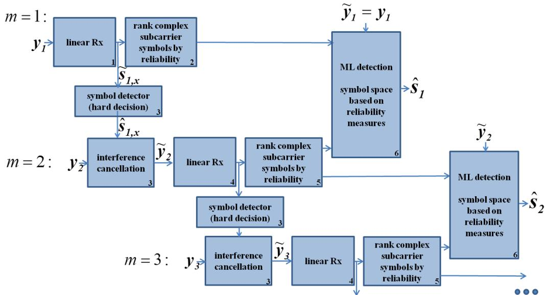
Fig. 2. ML based detector with linear preprocessing and interference cancellation for search space reduction
