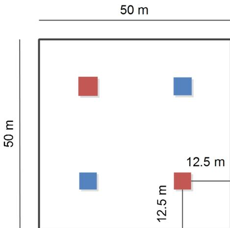
Fig. 1. Indoor inter-operator deployment scenario. Different colors represent base stations of different operators.
