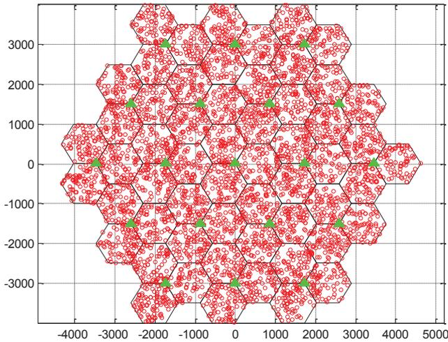
Fig. 1. Simulation scenario with 19 sites (57 cells).
