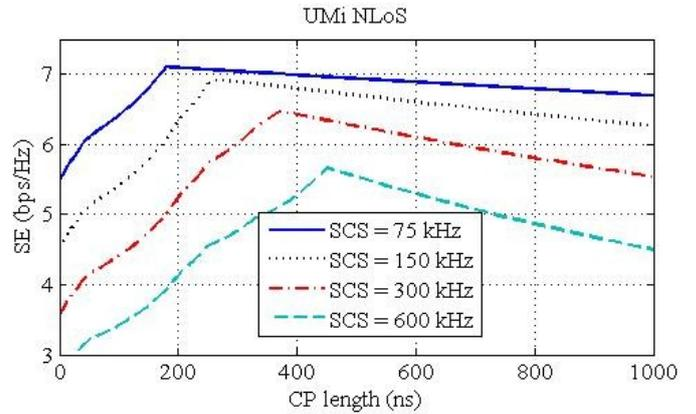
Figure 4. Spectral efficiency as a function of CP length; UMi.
