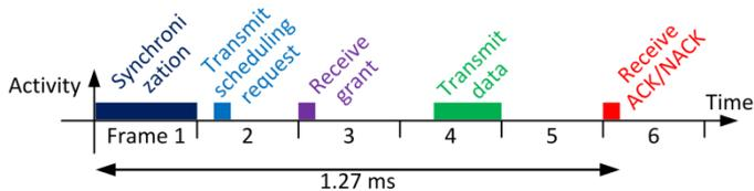
Figure 7. Procedure for UE initiated transmission in 5G.
