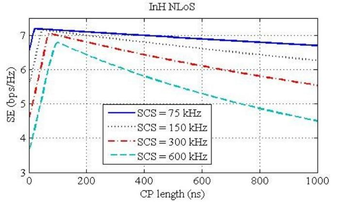
Figure 3. Spectral efficiency as a function of CP length; InH.
