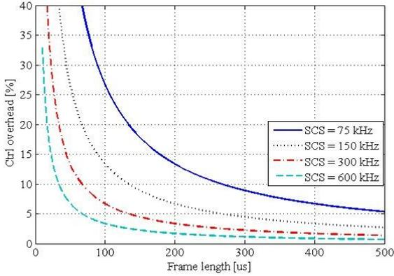
**Figure 5. Amount of control overhead vs. frame length.**
