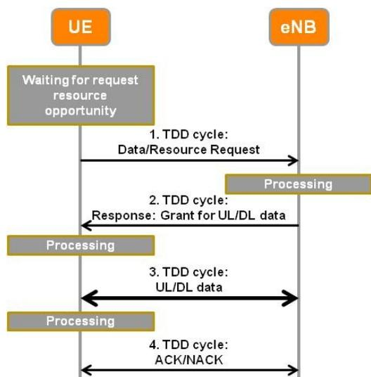
Figure 1. Required TDD cycles for UE initiated data traffic.
