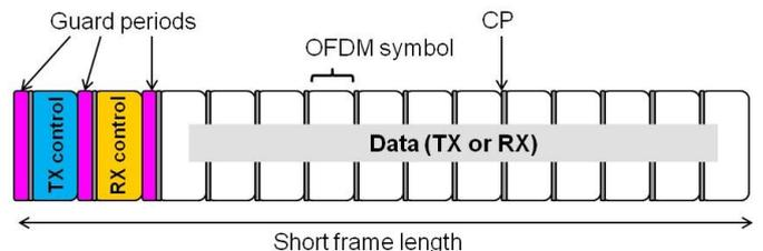
Figure 2. Proposed 5G physical frame structure.
