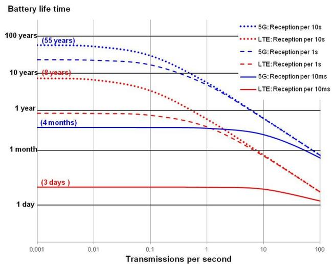
Figure 8. Battery life time comparison between LTE and 5G.
