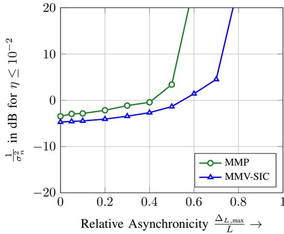
Fig. 6. Performance of the schemes under asynchronous transmissions in a setup with  $K = 100$  nodes,  $m = 15$  observations and a frame length of  $L = 1000$ . Per node activity probability is  $p_a = 0.35$
