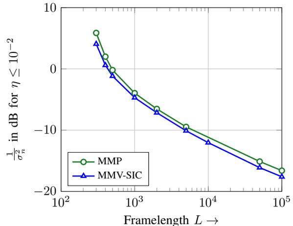
Fig. 4.  $\frac{1}{\sigma_n^2}$  required to meet an activity error rate of  $\eta \leq 10^{-2}$  for different frame-length  $L$ .
