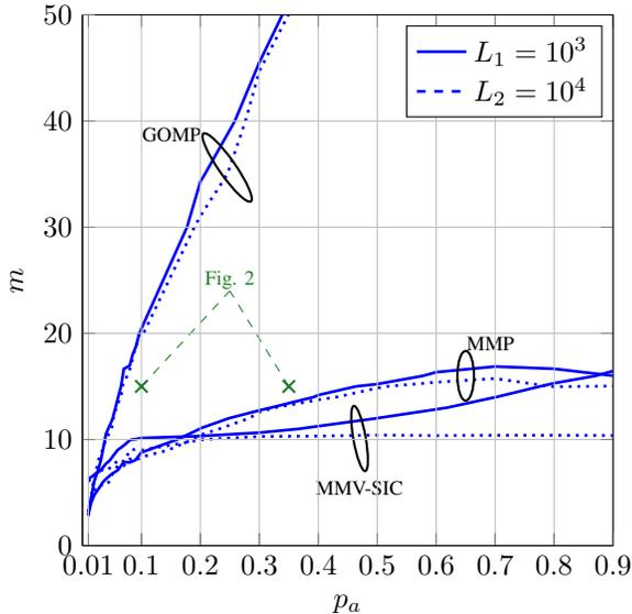
Fig. 3. Phase transition diagram for different frame length. The area above the curve denotes the tuples of  $m$  and  $p_a$  where the detector is able achieve an activity error rate of  $\eta \leq 10^{-2}$
